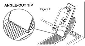
Angle-Out Tip: The sole plate has an angle-out tip at the back, this feature will prevent "dragging-off" the hot melt adhesive, especially in doorway situations where the iron is removed by angling it up and out.
